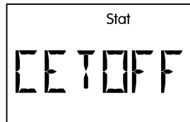
Collector - excess temperature - cutoff is active
