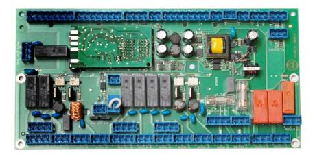
Power unit UVR 1611E-NP with processor module
