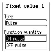
Select the **function quantity:** When activated, either an ON pulse (from OFF to ON) or an OFF pulse (from ON to OFF) will be generated, depending on the settings made here.
