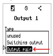
These outputs can be used as single switching outputs or as an output pair together with the following switching output (e.g. to control a mixer drive).
