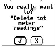
Answer the confirmation prompt by tapping either the tick ( ) (= Yes) or the cross ( ) (= No). After the deletion of the total meter readings, the current date will be displayed.
