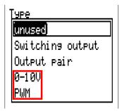
These outputs provide a voltage between 0 and 10 V, e.g. for output-dependent control of burners (burner modulation) or speed control of electronic pumps.
