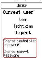
An **Expert** can change the passwords for Technician and Expert. A **Technician** can only change the Technician password.
