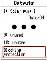
Circulating pumps which do not run for a long period (e.g. heating circuit pump during the summer) often encounter start-up problems as a result of corrosion. This problem can be avoided by starting the pump periodically for 30 seconds.
