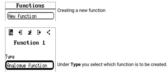
The line at the top of the "Function" menu provides access to **fiD** (type and designation), **input variables**, **parameters**, **output variables** and **links**.
