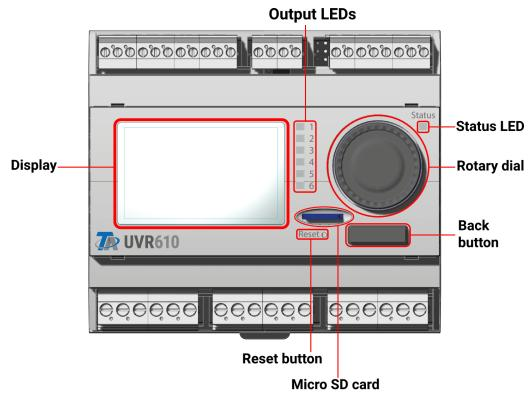
The **display** is used to navigate within the controller, to program functions, read in values, access other devices, etc.
