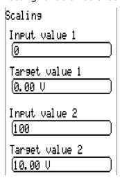
**Temperature value,** e.g. from an analogue function: Mode PWM, the temperature 0 °C should correspond to 0%, 100.0 °C should correspond to 100%:
