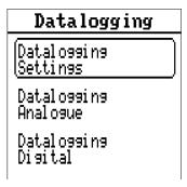
In this menu, the settings for datalogging are defined via CAN bus or on the SD card of the controller for analogue and digital values.
