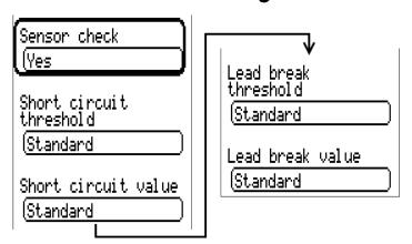
When "Sensor check" is active (setting: "Yes"), a short circuit or a lead break will automatically generate an error message.
