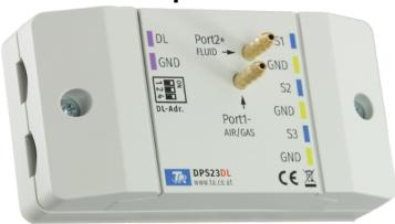
The **DPS23-DL** differential pressure sensor measures the pressure difference between the two ports. Alternatively, one of these ports can be left unconnected, in which case the differential pressure between the port and the module's immediate environment will be measured.
