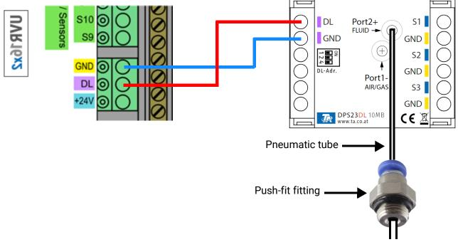
The principles of DL bus cabling are described extensively in the installation instructions for the free-ly programmable controllers. The polarity of the data link is interchangeable.
