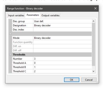
3 thresholds, defined in sequence from 0 to 2, correctly transfer the decoded value.
