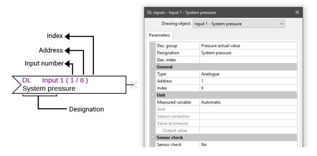
The most important settings can be found under **General**. Specify the DL bus address set on the DPS23-DL (default 1), as well as the index of the required input.
