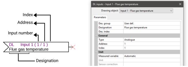
The most important settings can be found under **General**. Here, specify the DL bus address set on the UMV5-DL (default 1), as well as the index of the required input.
