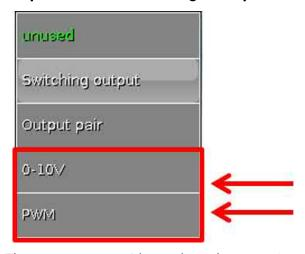
These outputs provide a voltage between 0 and 10 V, e.g. for output-dependent control of burners (burner modulation) or speed control of electronic pumps.
