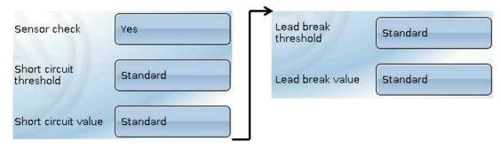
When "Sensor check" is active (setting: "Yes"), a short circuit or a lead break will automatically generate an error message: A warning symbol is displayed in the upper status line, and the defective sensor is shown with a red border around it in the "Inputs" menu.
