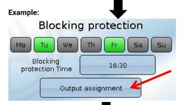
The outputs selected in the **Output assignment** will be switched on for 30 seconds on Tuesday and Friday at 4:30 p.m. if the output has not been active since the last controller start or since blocking protection was last initiated.
