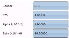
The R25 value is also required for the evaluation of PTC sensors. The nominal resistance R25 is based on 25 °C.
