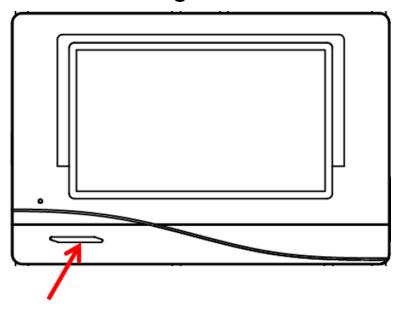
The indicator light can indicate a variety of statuses by means of three colours.
