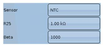
For evaluating the NTC sensors, the R25 value and the beta value must be specified.
