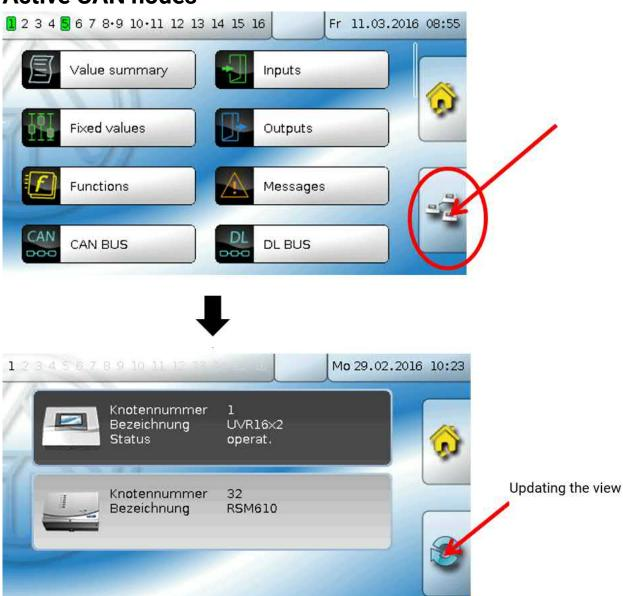
Tapping the button displays the active CAN nodes in the CAN bus network. "Status" displays the controller's CAN bus status. Following a controller start the status changes automatically, according to a predefined process, from  $init. \rightarrow preop(erational) \rightarrow operat(ional)$ . Only then is it possible to communicate with other CAN bus devices.
