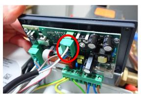
4. Plug enclosed cable to the new valve.
