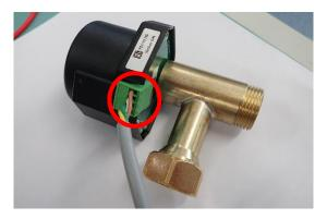
5. Route cable back through controller casing and fasten with cable tie. Plug new valve cable in the same spot on the electronics and screw front plate back on.
