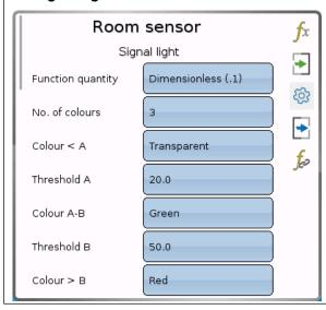
The signal light reflects the state of a value using a coloured icon on the main page. The signal light setting is similar to the range function: The number of thresholds (1-5) is selected and each threshold (as well as outside the limit thresholds) is assigned a colour. The measurement is monitored and the colour of the active threshold is visible on the main page.
