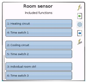
Under **Involved functions**, you can set the functions that should be shown. The first line of each pair of lines only displays valid functions (heating circuit, cooling circuit, individual room control, stage selector switch) that have already been programmed. Up to 3 of these functions are possible, even several of the same function type.
