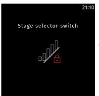
If the stage selector switch enable goes to OFF, the buttons are hidden and a lock appears in front of the bars.
