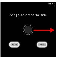
If the base stage is set to 0 and the maximum stage is set to 1, a digital ON/OFF switch is realised. In this case, the page for the stage selector switch has a button for switching on/off.
