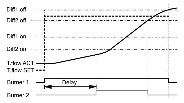
If there is demand (flow set temperature T.flow SET suddenly increases) and the flow temperature is less than the switch on temperature of the controlling boiler (=T.flow SET + DIFF1 ON), the first demand is generated. If the flow temperature remains under the switch-on temperature for the second boiler (T.flow SET + DIFF2 ON), a second demand is generated. The boilers are switched off in the same sequence as the flow temperatures exceed the switch-off temperatures (T.flow SDET + DIFF OFF).
