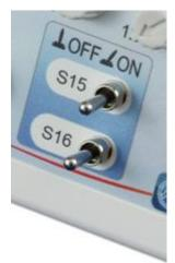
Using the two **changeover switches** for **inputs 15 and 16**, these inputs can be simulated as analogue temperature inputs or digital inputs, **depending on programming**.
