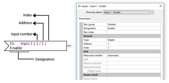
The most important settings can be found under **General**. Here, specify the DL bus address set on the DI5-DL (default 1), as well as the index of the required input.
