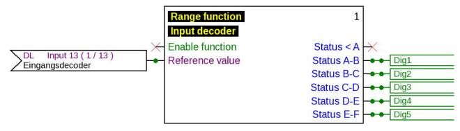
The DL input with **Index 13** issues a number between 0 and 31, which is decoded by the binary decoder to produce a binary number with the input statuses. That DL input must therefore be linked to the input variable **Reference value** (as shown in the graphic).
