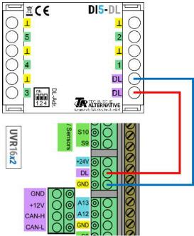
The principles of DL bus cabling are described extensively in the installation instructions for the freely programmable controllers. The polarity of the data link is interchangeable.
