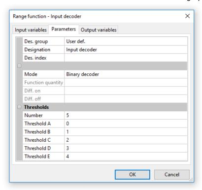
5 thresholds, defined in sequence from 0 to 4, correctly transfer the decoded value.
