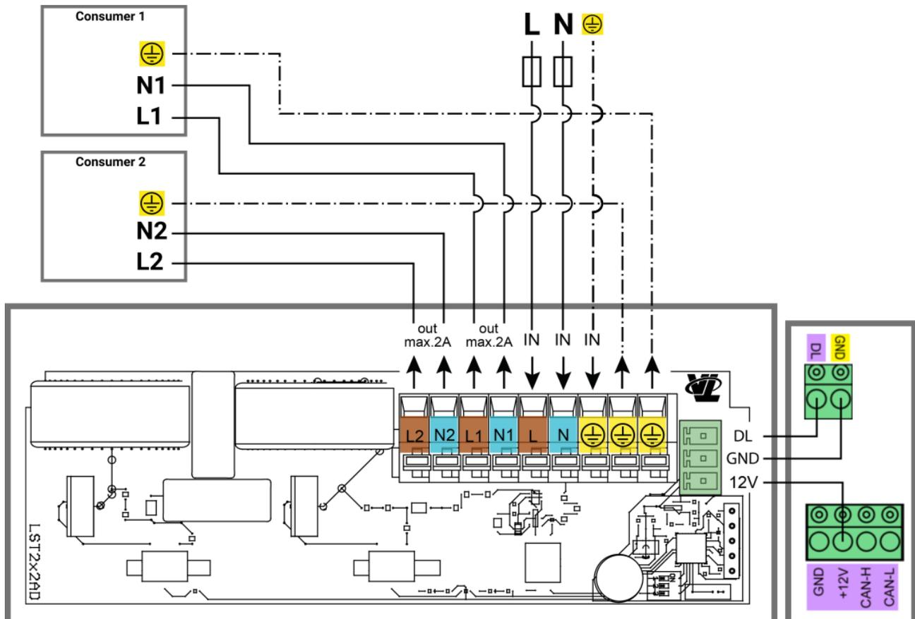
Mind the usage of suitable wire sizes and temperature resistance according to applicable norms.
