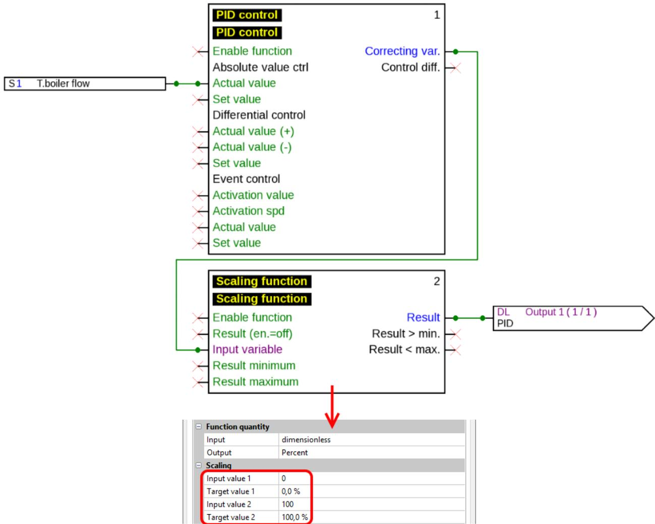
In the scaling function, a PID correcting variable of e.g. **60** results in **60.0%**.
