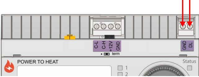
Devices connected via CORA-DL do not affect the DL bus load.
