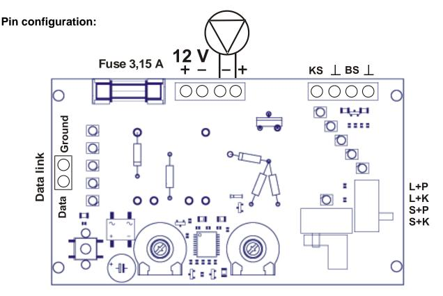
When using the master-slave function, the data link must be connected in-phase to both units (data to data, ground to ground).
