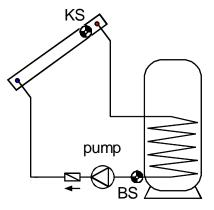
The pump runs when sensor **KS** has a temperature of *diff* higher than sensor **BS** and **BS** has not exceeded the threshold *max*.
