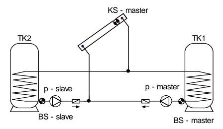
• **2-pump mode:** as can be seen in the schematic diagram, a pump is connected to both master and slave. The master pump has absolute priority, hence the slave pump can only be switched on if the master pump is switched off (dependent on the starting conditions). 2-pump mode is activated if the terminals of the collector sensor at the slave remain disconnected (= interruption).
