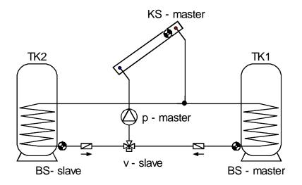
• **Pump-valve mode:** the common pump is connected to the master controller, the slave controls the valve. As soon as the starting condition is no longer fulfilled at the master, the slave receives the command to switch on the pump and switches the valve to "its" consumer TK2. Pump-valve mode is activated if the terminals of the collector sensor at the slave are bridged with a jumper (= short circuit).
