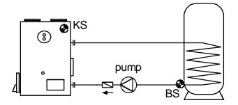
The pump runs when **sensor KS** is greater than the threshold **max** (here used as "min") and **sensor KS** is greater than **BS** by the difference **diff**.
