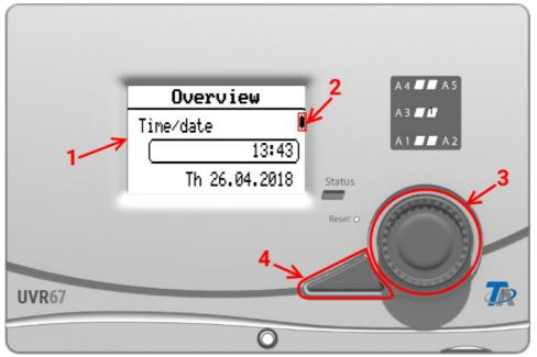
The display (1) on the front shows information about sensor values, menu position, parameterisation, etc.
