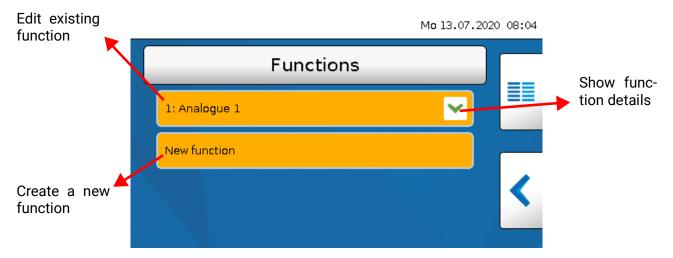
You can choose from **43** different functions and create up to **128** functions. Functions can also be created multiple times.
