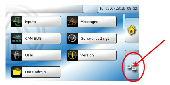
Tapping the button displays the active CAN nodes in the CAN bus network.
