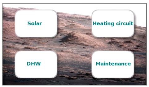
If you press the background image for 3 seconds, 4 buttons appear which enable access to the version information of the CAN monitor, the general settings or the date, time and location settings, and the main menu of the CAN monitor.
