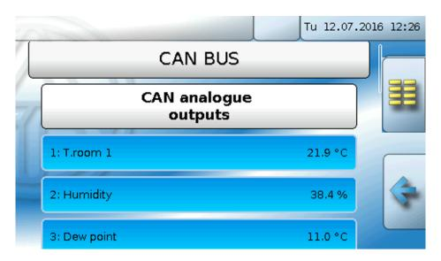
As there are no other analogue values available as the source for CAN analogue outputs, no instructions are given here for programming other CAN analogue outputs.
