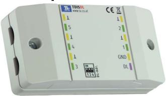
The **TDI5-DL** (Temperature and **D**igital Input) translates up to five signals for the data link (DL bus), which can be either a digital signal (On/Off) or the measurement from a PT1000 sensor. **Digital signals must be potential-free. Please note:** Due to the inertia of the DL bus, this module is **not** suitable for time-critical applications (e.g. digital inputs as pushbuttons).
