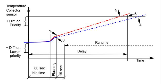
The device monitors the collector temperature while the lower priority consumer is being charged. If, while the pump is running, the collector temperature once again reaches the **start** differential (collector – reference) for the consumer **currently** being charged, the priority timer will be activated. If a radiation sensor is being used, the radiation level must exceed a threshold value, instead of the temperature differential.
