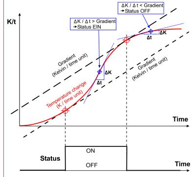
The status switches to ON if the rise in temperature **within a tenth** of the set time unit is greater than the set gradient.
