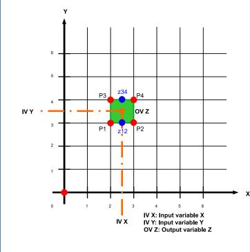
To calculate the Z value, firstly the 2 average values between P1 and P2 (z12) and P3 and P4 (z34) are calculated. Those two average values z12 and z34 are then averaged in turn and the resulting value is issued as the Z output variable.
