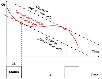
The Status switches to ON at the point where the curve of the **Temperature change** becomes steeper than the gradient.
