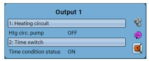
In this example, output 1 is controlled by two functions, and it has just been switched on by function 2 (Time switch).
