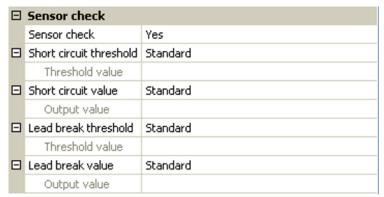
In order to make good use of the sensor check, the short circuit and lead break thresholds should be changed from "Standard" to "**User defined**" and the required threshold values defined. The required short circuit and lead break values will subsequently also be defined by the user.
