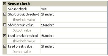
If the **Standard** thresholds are selected, a short circuit will be indicated if the value falls below the **measurement limit** and a lead break will be indicated if the value exceeds the **measurement limit**.
