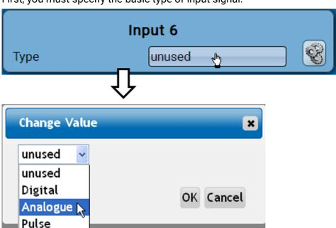
Then select the measured variable. For the measured variable "Temperature", you must also define the **sensor type**.
