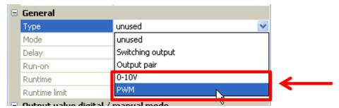
These outputs provide a voltage between 0 and 10 V, e.g. for output-dependent control of burners (burner modulation) or speed control of electronic pumps.
