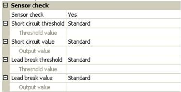
If the **Standard** thresholds are selected, a short circuit will be indicated if the value falls below the **measurement limit** and a lead break will be indicated if the value exceeds the **measurement limit**.
