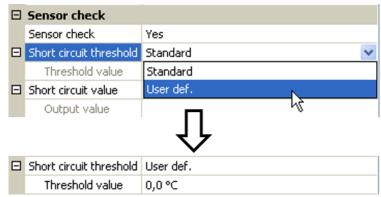
By selecting suitable thresholds and values for short circuit and lead break, a fixed value can be specified for the module in the event of sensor failure at the transmission node, to allow a function to continue operating in emergency mode (fixed hysteresis: 1.0 °C).
