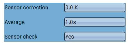
When "Sensor check" is active (setting: "Yes"), a short circuit or a lead break will automatically generate an error message: A warning symbol is displayed in the upper status line, and the defective sensor is shown with a red border around it in the "Inputs" menu.
