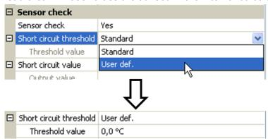
By selecting suitable thresholds and values for short circuit and lead break, a fixed value can be specified for the module in the event of sensor failure, to allow a function to continue operating in emergency mode (fixed hysteresis: 1.0 °C).
