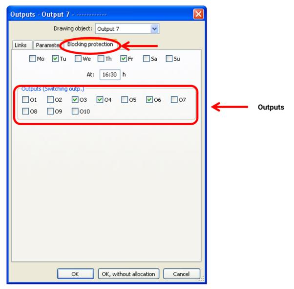
In this example, the pumps 3, 4 and 6 will be run for 30 seconds on Tuesday and Friday at 16:30 h if the output has not been active since the module was started or since blocking protection was last initiated.
