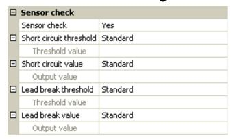
If "Sensor check" is active (setting: "Yes"), a short circuit or a lead break will automatically generate an error message: A warning symbol is displayed in the upper status line, and the faulty sensor is shown with a red border around it in the "Inputs" menu.
