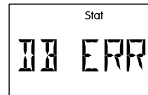
Drain-back low water
