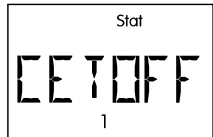
Collector - excess temperature - switch-off is active
