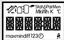
The factory setting is loaded by pressing button during plugging in. The following appears on the display: (Load factory setting)
