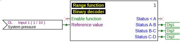
The DL input with **Index 13** outputs a number between 0 and 7, which is decoded by the binary decoder to produce a binary number with the input statuses. That DL input must therefore be linked to the input variable **Reference value** (as shown in the graphic).
