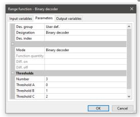
3 thresholds, defined in sequence from 0 to 2, correctly transfer the decoded value.
