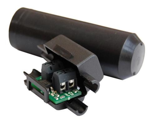
The AC/DC converter was invented for 230VAC signal detection in conjunction with the UVR control units. An external 230VAC signal from UVR control units can be detected using this sensor. To do so, the control unit's sensor input has to be set to "Digital". If the terminals of the AC/DC converter are subject to 230VAC, the controller displays ON. The controller displays OFF when there is no voltage.
