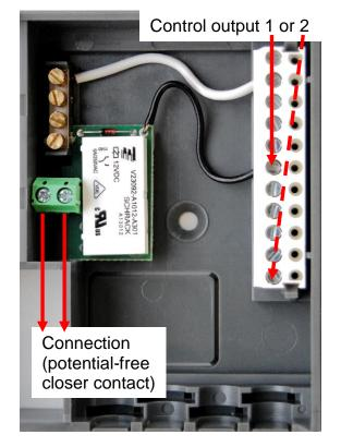
The relay module is connected to the sensor earth and a control output in accordance with the above images. The 4-pole earth strip is enclosed for the ESR31 controller.
