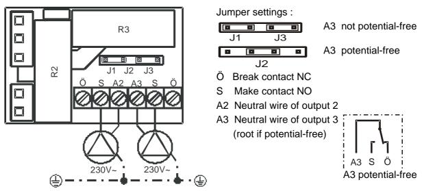
Output **A3** can be made potential-free by means of the **jumpers** (J1 to J3). To do so, jumper **J2** is placed instead of J1 and J3 (standard), while connection A3 is the root.
