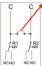
**Drilled hole**: The relay contacts are - without connection x) - potential-free, for which both roots(C) have been connected at the factory. Widening the hole between both relays to at least 6 mm in diameter separates the potential of both outputs across each other in accordance with industry
