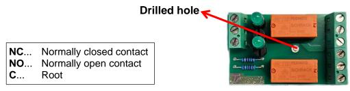
The auxiliary relay can be connected across any two analogue outputs if these are programmed as switching outputs.
