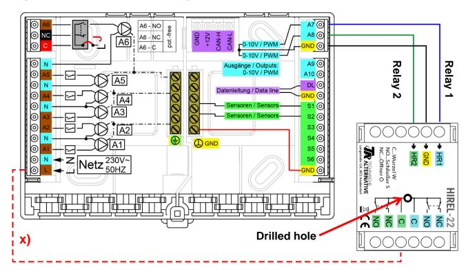
**X)** This connection enables the HIREL22 relay contacts to switch the phase conductor (230 V) to become conductive. As a consequence the relay outputs are no longer potential-free.
