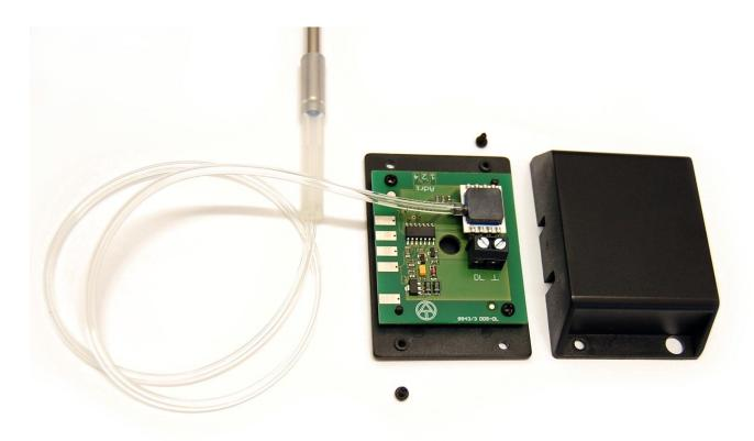
The differential pressure sensor DDS-DL is based on the principle of two silicon membranes rotated at 90° relative to each other so that they deflect under the differential pressure. The ohmic resistance which changes as a result of the deflection is captured as the measured variable. The displacement of the membranes relative to each other guarantees, even at the least pressure, position-independent signal accuracy.
