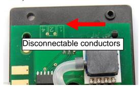
The **address** is specified on the adapter by breaking the conductors which are labelled (1), 2 and 4. These are located on the short PCB side close to the actual pressure sensor. If none of the conductors are cut, the adapter is assigned address 1 (factory setting). Provided no other sensors are connected to the DL-bus, no change of address is required.
