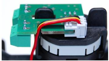
The supplied ribbon cable is connected to the volume flow sensor FTS....DL (as per the figure) and the pressure sensor. The plugs are not interchangeable.
