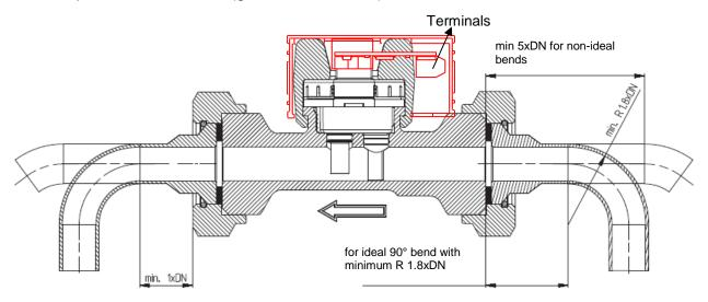
The flow direction must be observed without fail (indicated on the sensor by an arrow). The fitting position can be freely selected.
