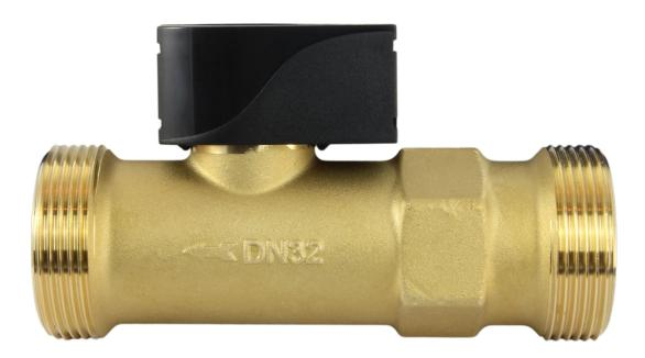
FTS...DL electronic volume flow sensors have a measurement principle based on Karman vortex streets. The generation of eddies from an obstructing body projecting into the flow is strictly proportional to the flow velocity. The generated eddies are detected by a piezoelectric paddle and evaluated by the integrated electronics. A microprocessor converts the analogue measurement values into a serial digital signal suitable for the DL bus (data link).
