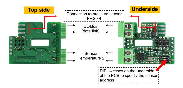
The polarity of the connections ("earth") is interchangeable, hence is unimportant.
